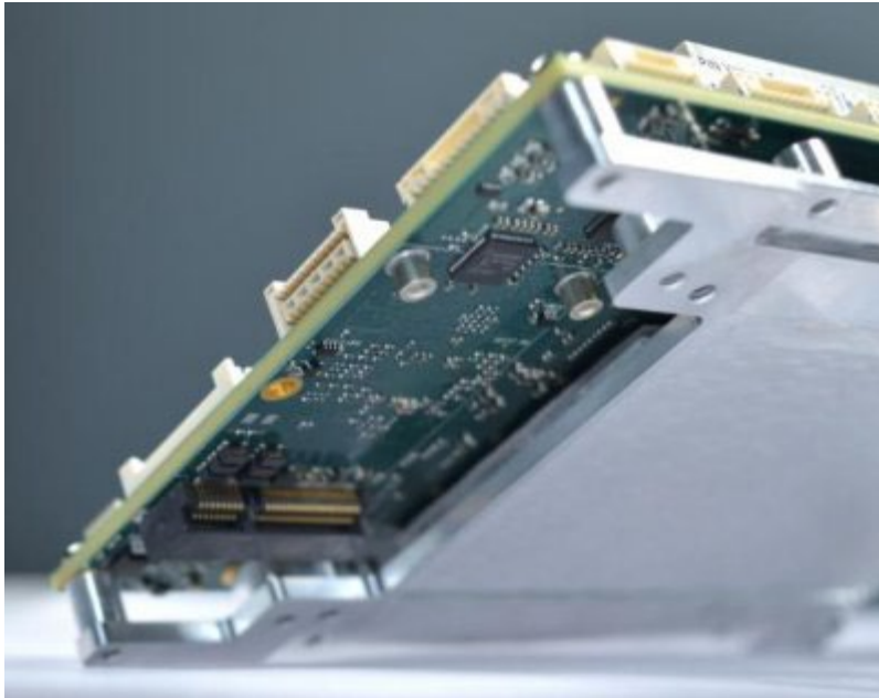
Second half/full-size MiniCard socket available on bottom side
