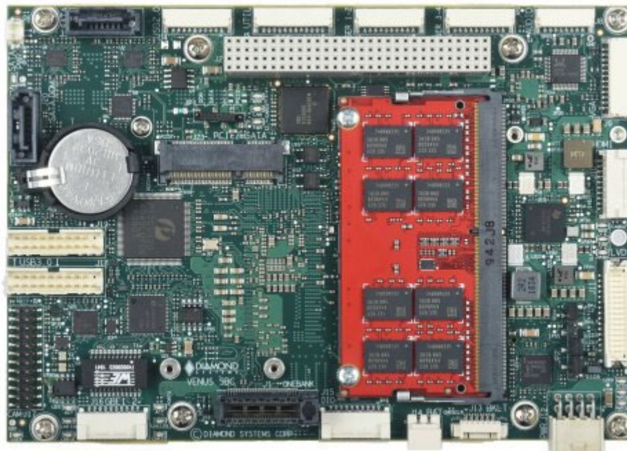
Diamond's unique rugged RSODIMM memory module installed on Venus
