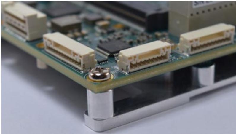
Thicker PCB inhibits flexing from high vibration
