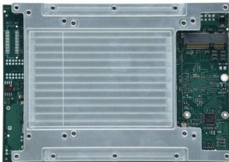
Heat spreader on bottom side
