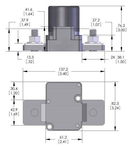
**Power Terminals** Zinc Plated M12 X 1.75 Bolt Stainless M12 X 1.75 Flanged Nut
