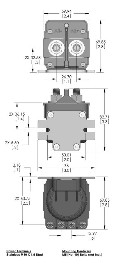
Power Terminals Stainless M10 X 1.5 Stud Stainless M10 X 1.5 Flanged Nut
