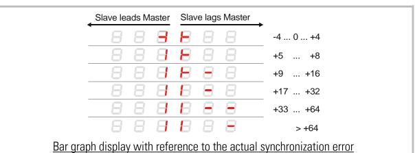
The diagram shows positive errors only (Slave lags Master). Negative errors are mirror-inverted.
