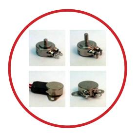
Precision temperature accuracy and long life reliability are achieved through the use of the well known Klixon® snap–acting disc. This unique mechanism multiplies the motion of the temperature sensor and actuates a switch capable of handling high power. Welded closed after accurate calibration, the M2 is tamperproof.
